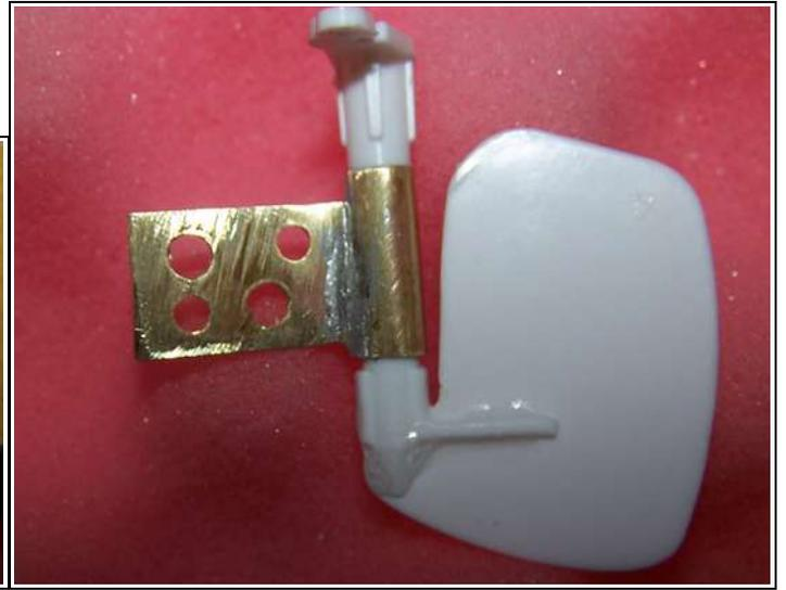
Marked the location on the back of the Hobbyzone float ensuring the control arm would move freely above the float. Used a hobbyknife to cut a slot into the foam and plastic float bottom.
