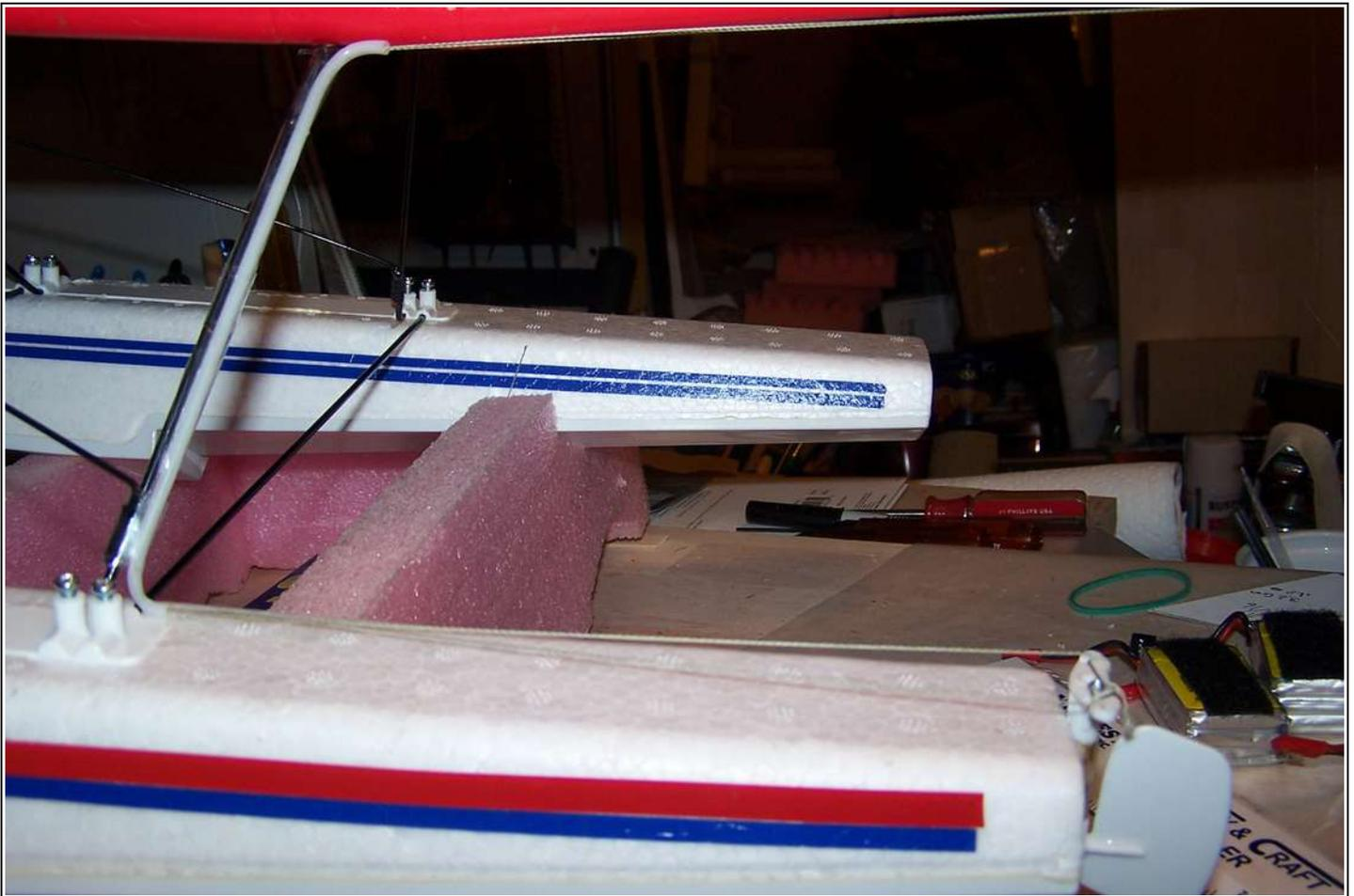
A single small screw in the water rudder control arm allows adjustment on the pull-pull lines. This has worked very well on my Flyzone Beaver and it works just as well on the Pilatus PC-6 and Sport Cub.
