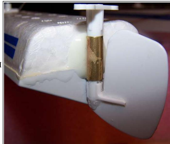
Inserted the adapter flange into the foam and glued with CA. Then added some epoxy with microballons. Used a pull-pull system to control the water rudder on my Multiplex Pilatus PC-6 similar to the mods I made on the Flyzone Beaver. Later adapted to my Parkzone Sport Cub with Hobbyzone Floats
